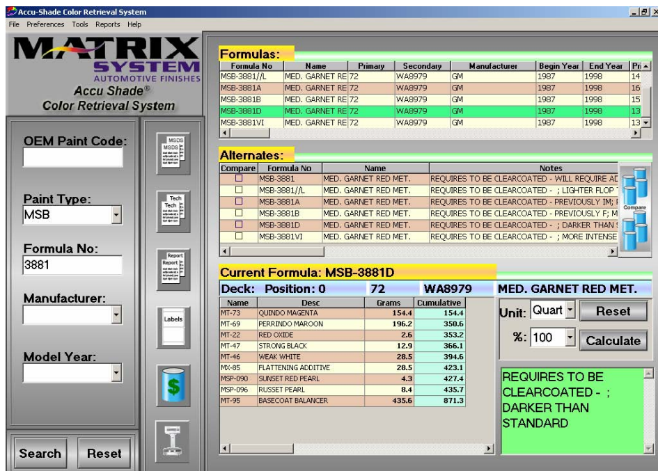
Figure 2 illustrates the alternate color formula MSB-3881D, notice the notes field in the lower right hand corner indicates "DARKER THAN STANDARD"
