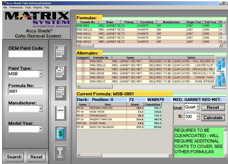
Figure 1 illustrates the standard color formula for MSB-3881, notice the notes field in the lower right hand corner indicates "SEE OTHER FORMULAS"
